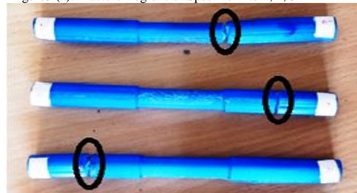
Figure5 (b): Fracture Regions of Specimen No 4, 5, 6
