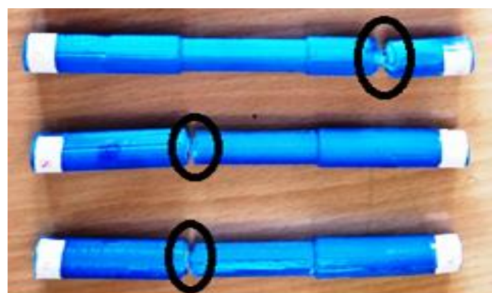
Figure5(c): Fracture Regions of Specimen No 7, 8, 9
